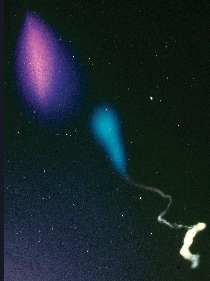
The cloud in the upper left hand part of the image is due to a barium release. The purple-red part is the ionized component which has become elongated along the Earth's magnetic field lines. The purple-blue cloud that surrounds the red ionized barium is a combination of the neutral barium and strontium. The blue and white trail in the lower portion of the image is from a TMA vapor trail that reveals the neutral wind trails as a function of altitude.
